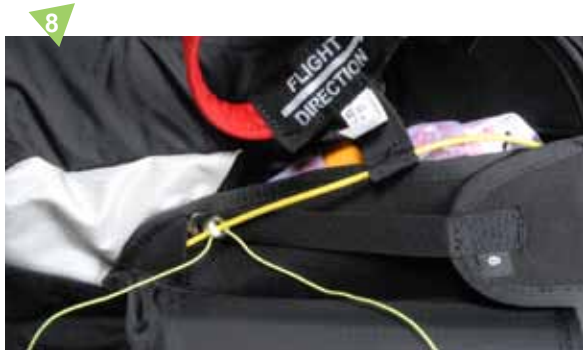
8 Push the handle's yellow cable ( rear section ) through the elasticated line and delicately remove the cord.
