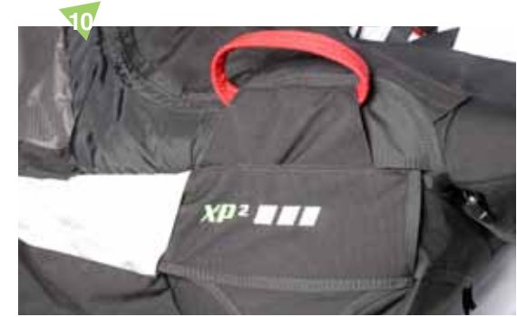
10 Fold the Cordura flap over the handle and insert it underneath the handle's flap to fasten it to the velcros.
