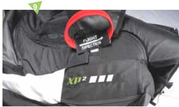
9 Close the Cordura flaps over the cable and push them through to the pocket's top lid .
