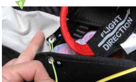
6 Push the end of the cord through the elasticated loop #4, then guide it through the grommets #5 and #6
